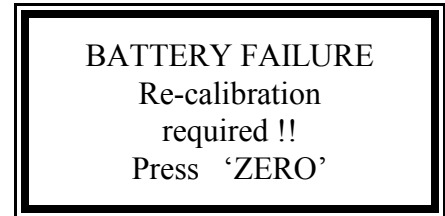
Figure 2-4 Message that appears when batteries must be replaced, or when the instrument is reset after new batteries are installed
