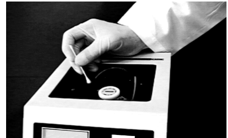
Figure 4-1 Cleaning the sample injection port before injecting a sample
